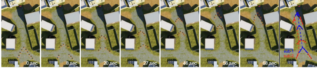
(b) A team of ten robots in a wedge formation traverses a progressively narrowing corridor between buildings.
