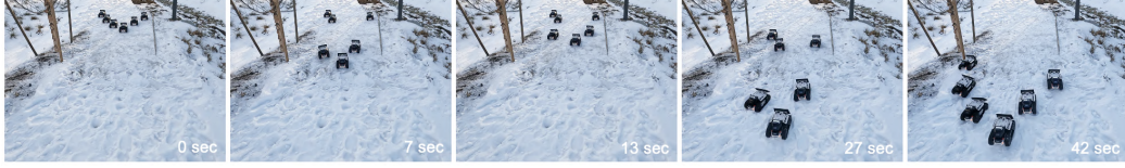
(b) A team of six robots in a wedge formation navigates through a forest-like environment with narrow corridors surrounded by scattered trees and obstacles.
