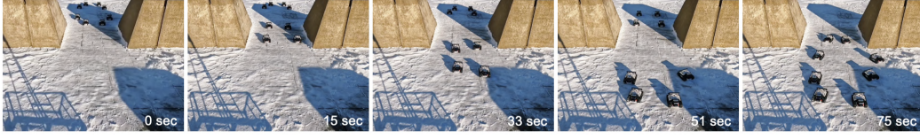
(a) A team of eight physical Limo robots with a circle formation traverses a narrow passage between two concrete security bollards.
